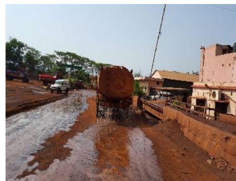
PHOTO-6 : SHOWING MOBILE SPRINKLERS INSIDE MINES
