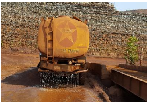
PHOTO-6 : SHOWING MOBILE SPRINKLERS INSIDE MINES
